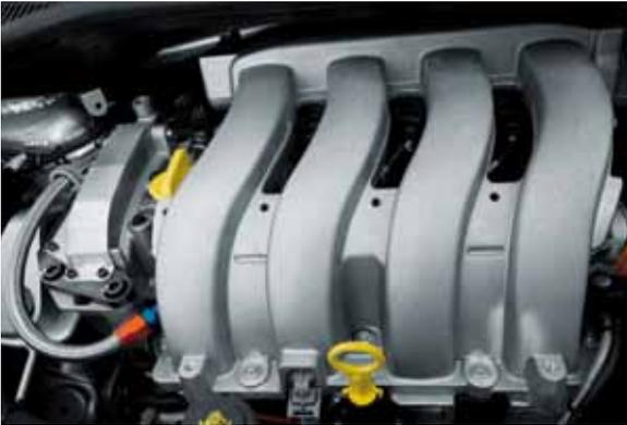
The main changes concern the pistons, camshaft, flywheel, exhaust system and the addition of a specific air box. This special preparation garners the engine an extra 33bhp compared with the production model, reaching a mighty 160bhp (118kW) of power at 7,000rpm. Maximum torque (180Nm) is reached at 5,500rpm.
